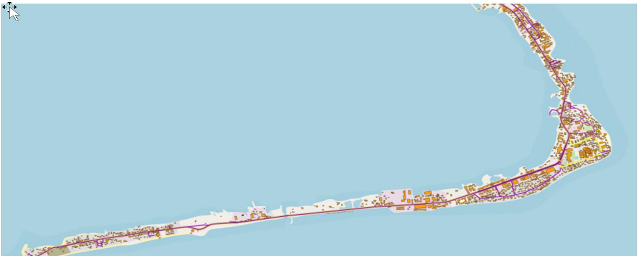
Figure 1 - Partial map of Majuro highlighting the main communal network path for the new fiber network. The fiber will be built along all main roads.
