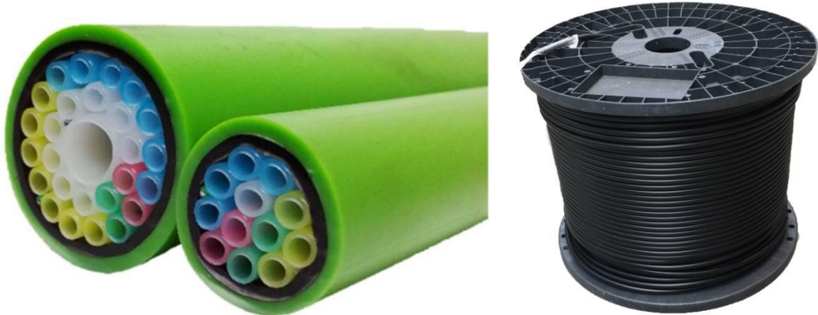
Figure 25 - Hexatronic Tight Protected Microduct products as examples. On the left are the Ribbonet products with the larger duct having 26 5/3.5mm ducts for individual premises and a single 12/10mm duct for feeder or core fibre. The overall duct is 38mm in diameter resulting in a low impact installation compared to traditional ducting. The drum on the right is a 500m drum of
